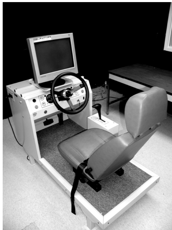
Passenger vehicle driving simulator driver's position
